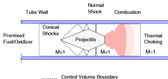
Fig. 1. Thermally choked ram accelerator propulsive mode.
