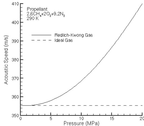
Fig. 4. Variation of  $2.6\text{CH}_4+2\text{O}_2+9.2\text{N}_2$  acoustic speed with pressure at 290 K.
