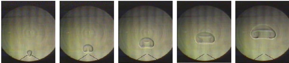
Fig .1. Flame development in a mixture 5.25% CH<sub>4</sub>. Square tube 250mm × 250mm × 800mm. Time interval between frames 0.08 sec.
