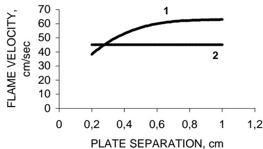
Fig. 6. Velocity of a downward propagating flame in stoichiometric methane/air mixture as a function of plate separation [8].
