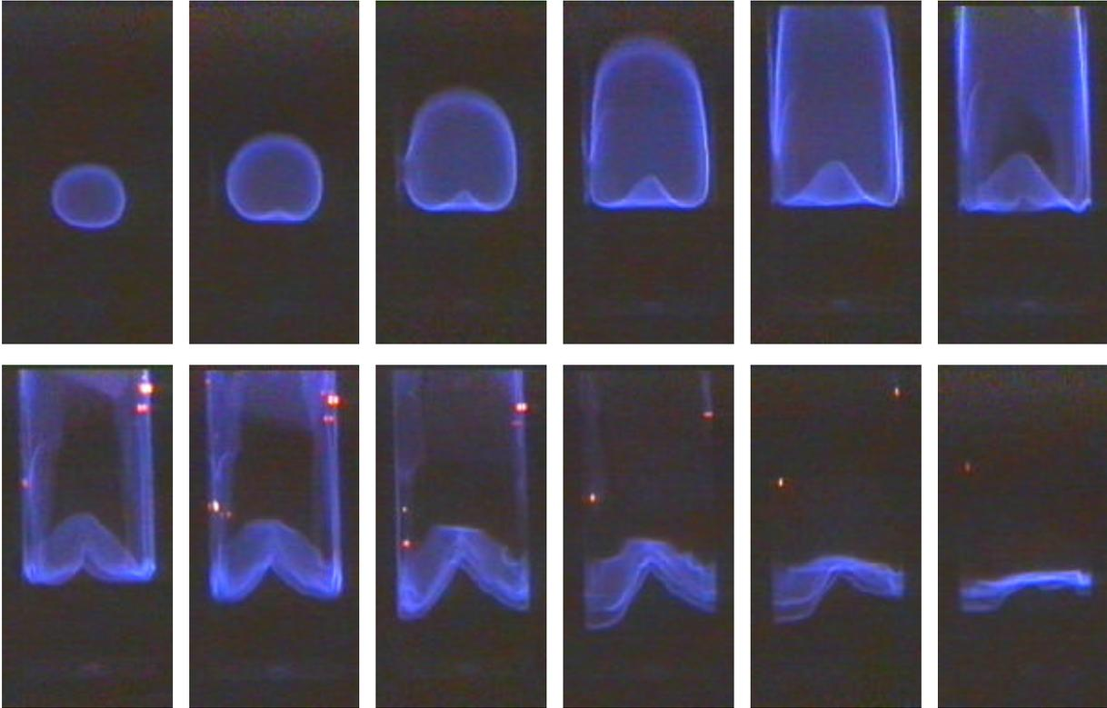
Fig. 4. Combustion developments from ignition to a plain downward propagating flames in a mixture 5.85% CH<sub>4</sub>. Square tube 250mm × 250mm × 800mm. Time interval between frames 0.06 sec
