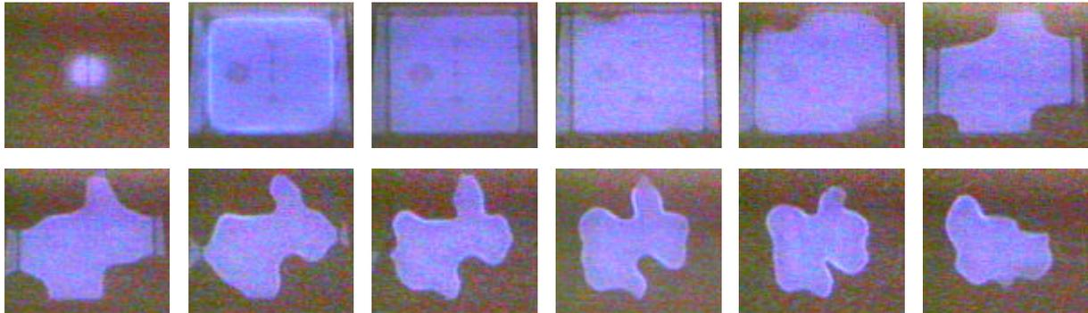
Fig. 5. Quenching process of a plain limit flame, propagating downward in 2.2 C<sub>3</sub>H<sub>8</sub> mixture, observed in a mirror located at the bottom closed end of the tube. Square tube 125mm × 125mm × 500mm Time interval between frames 0.2 sec
