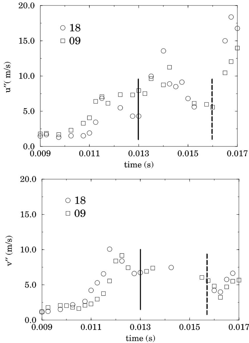
Figure 2. Temporal variations of  $u''$  and  $v''$  velocities at 9 and 18 mm along the 515 mm plane. The vertical lines indicate the arrival of the flame at the respective locations.
