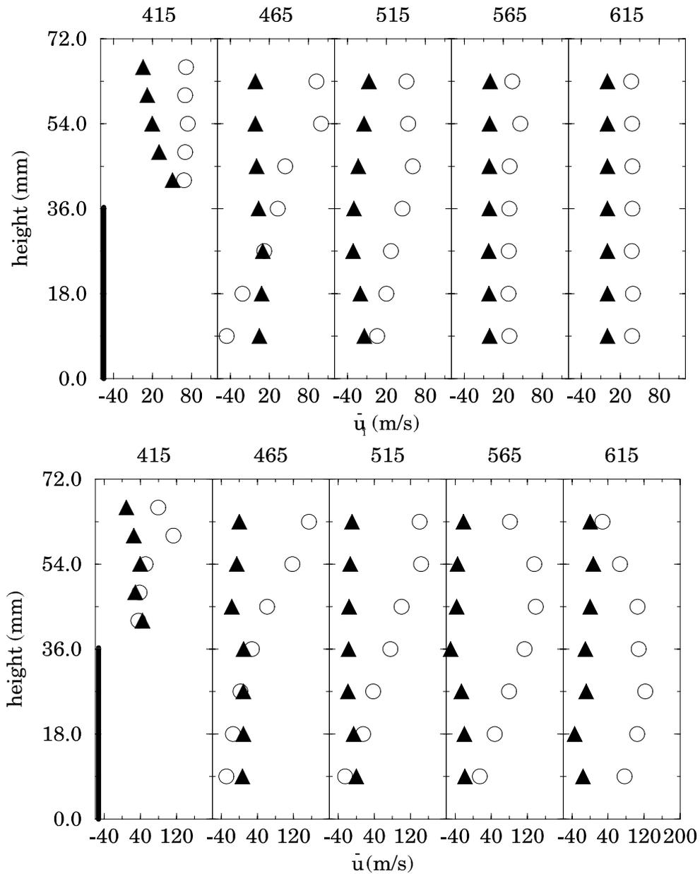
Figure 1. Spatial variations of mean velocities at the 415, 465, 515, 565 and 615 mm planes from the jet exit at (top) 11 ms and (bottom) 13.5 ms. The circles and triangles indicate axial and perpendicular velocity components respectively.
