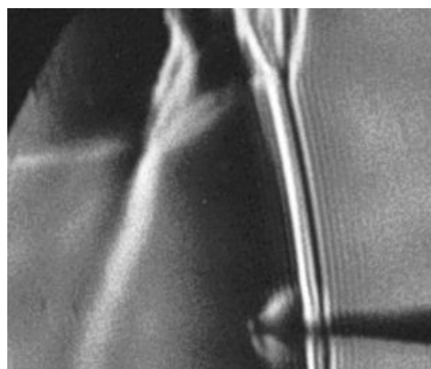
Fig. 3: Maximum observed fringe distance in front of the detonation front: 0.3 mm 2\text{H}_2 + \text{O}_2 + 2\text{Ar} initial pressure 5.8 kPa cell size \lambda 40.8 mm original section width 16.8 mm
