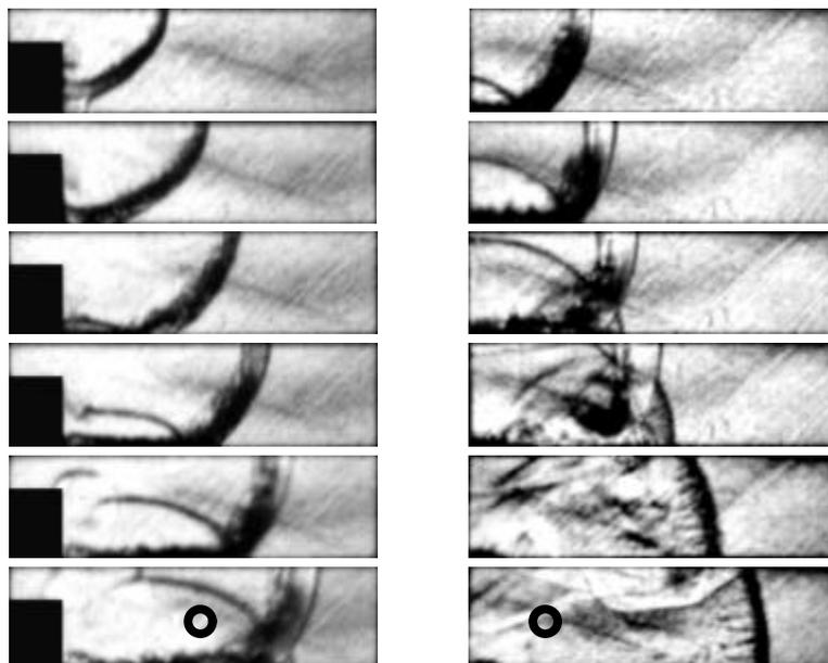
Fig.1 Schlieren photographs for  $p_0=53.3\text{kPa}$  and  $\beta=0$ . Circles denote the position  $D=65\text{ mm}$ .
