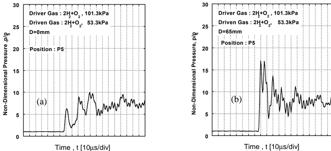
Fig.3 Pressure variation behind the step (a)  $D=0$  mm and (b)  $D=65$  mm for  $p_0=53.3\text{kPa}$  and  $\beta=0$ .
