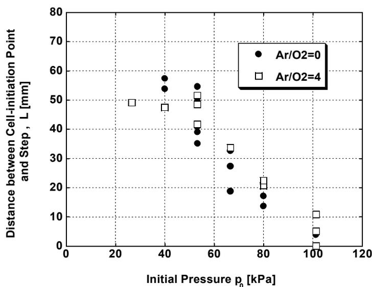
Fig.4 Relation between the re-initiation distance  $L$  and the initial pressure of the mixtures.
