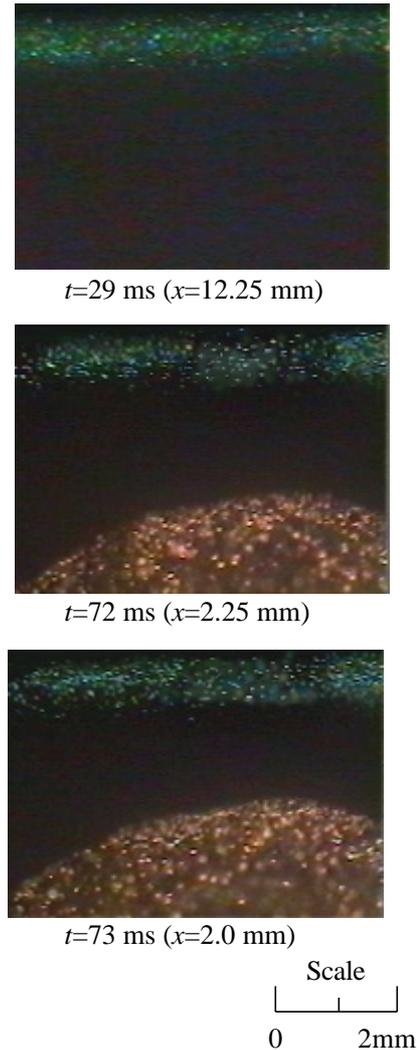
Fig. 3 Series of photomicrographs. 1,000 frames/s,  $t$ : time from ignition
