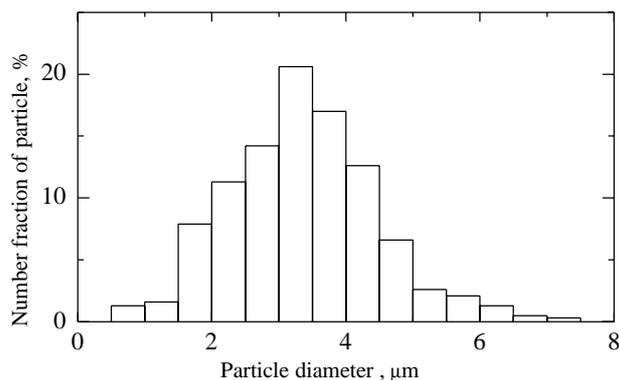
Fig. 2 Diameter distribution of iron particles.
