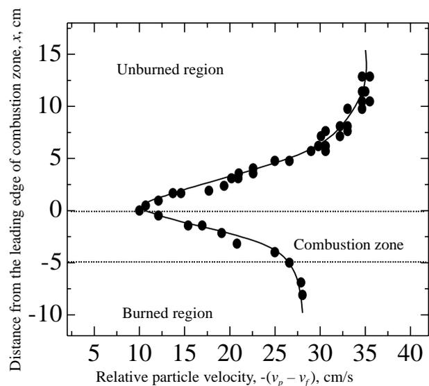
Fig.5 The relative velocity distribution of particles to the leading edge of combustion zone.
