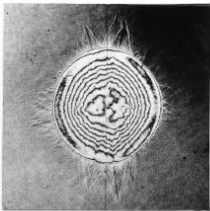
(f) 60kPa H_2/N_2 , 10mg explosive with SiO_2 powder
