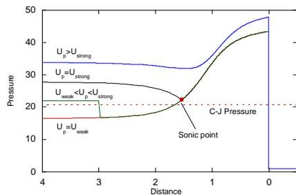
**Figure 1:** Steady ZND pressure profiles for different piston velocities ( $Ea_1=22$ ,  $Ea_2=35$ )
