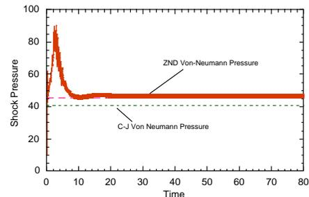
**Figure 2:** Stable pathological detonation with blast initiation ( $Ea_1=22$ ,  $Ea_2=35$ )
