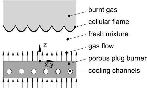
Figure 1: Burner geometry
