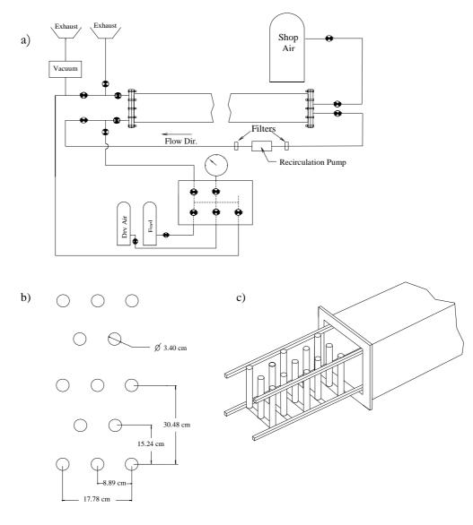
Figure 1: a) schematic of gas handling system b) plan view of obstacle arrangement c) 3-D view of obstacle-tube assembly
