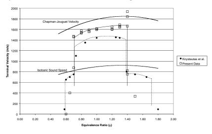
Figure 4: Terminal steady state velocities of propane-air at different equivalence ratios.
