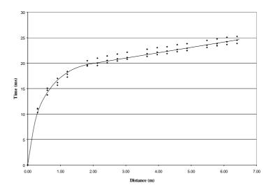
Figure 2: x-t diagram of flame arrival times for stoichiometric methane-air for repeated shots
