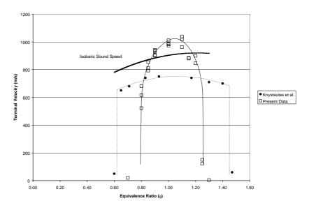
Figure 3: Terminal steady state velocities of methane-air at different equivalence ratios.
