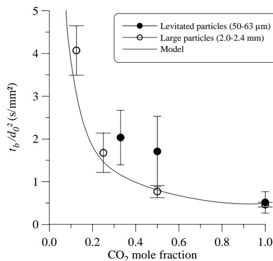
**Figure 6** Comparison of measured burning times of levitated Mg particles in CO<sub>2</sub> and CO<sub>2</sub>/Ar mixtures with data for large particles [4] and with predictions by model [5]
