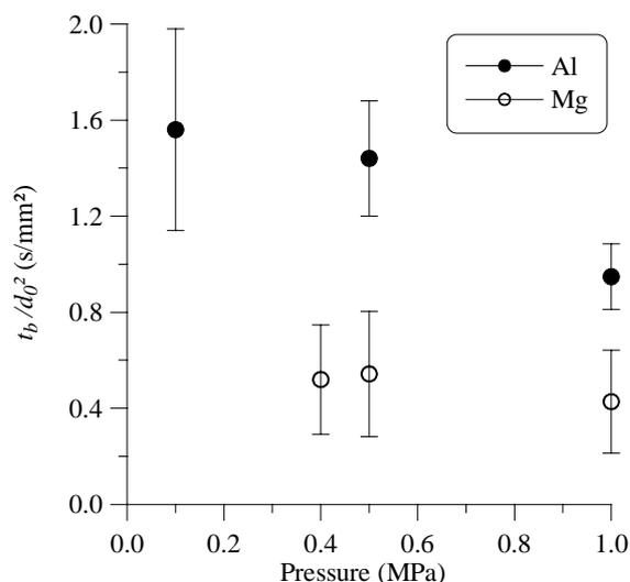
**Figure 5** Effect of pressure on the inverse burning rate of Mg and Al particles in CO<sub>2</sub> ( $t_b$  is the burning time,  $d_0$  is the initial size)
