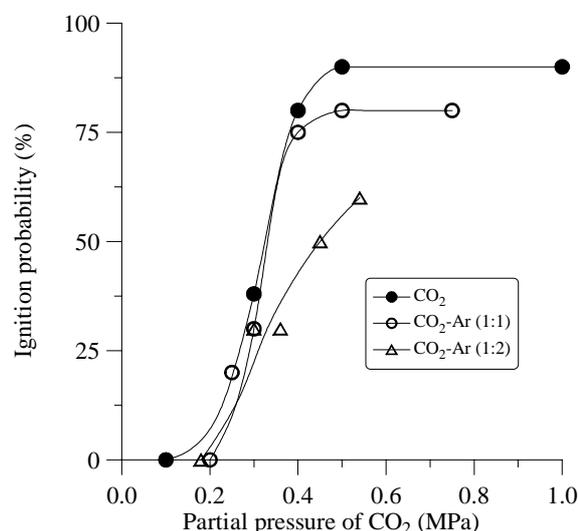
**Figure 2** Ignition probability of spherical Mg particles (50-63 μm) in different CO<sub>2</sub> - Ar mixtures versus partial pressure of CO<sub>2</sub>
