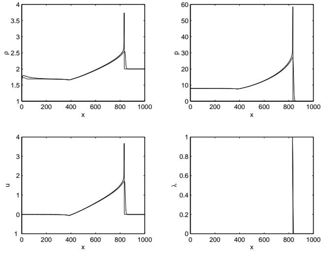
Figure 1: Plot of the DNS ( $\Delta x_{DNS} = 0.2mm$ ) and PB ( $\Delta x_{PB} = 4.0mm$ ) solutions for cylindrical geometry.
