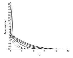
At  $t_{ch} > t_{ig}$ , the kinetic mode of ignition is observed. The gaseous suspension is ignited at the equal temperature of the gas and the particles, *i.e.* the process can be described by an uni-temperature model (Fig. 2). Kinetic-controlled (one-temperature) regime of ignition
