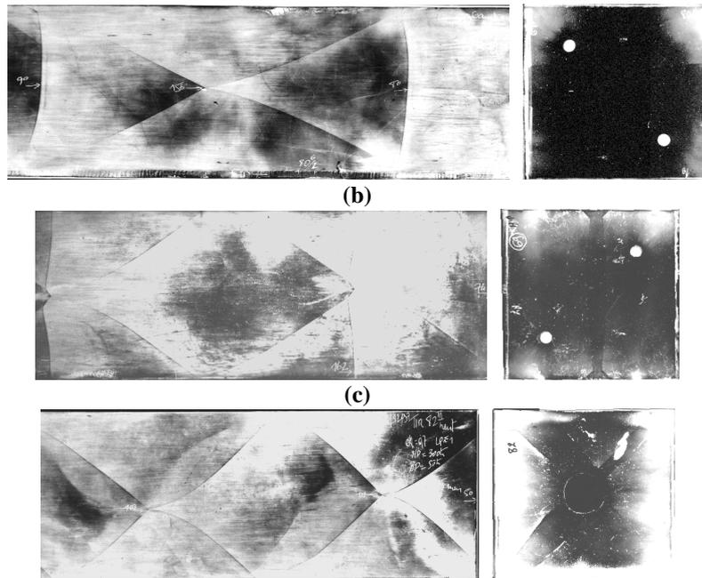
Fig. 1: Three types of multidimensional structures recorded on soot plates. Structure with slapping waves, rectangular type, (a) in phase and (b) out of phase, and structure without slapping waves, (c) diagonal type.
