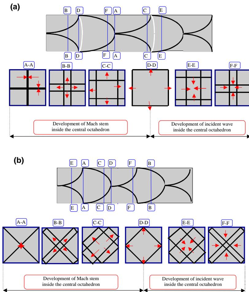
Fig 2: Schematic diagram of the front shocks at different locations of the cycle of the detonation cell. (a) Rectangular Ra and (b) diagonal D mode detonation cell. The arrows show the motion of the triple point lines.
