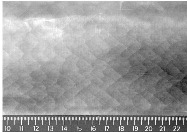
Fig.2 - Soot-plate record of the detonation in hydrogen-air mixture ( $r=0.87$ ) with aluminium particles F (flakes,  $\sigma=220\text{g/m}^3$ )
