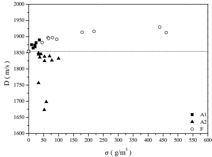
Fig.1 - Detonation velocity versus mass particle concentration for different aluminium particles
