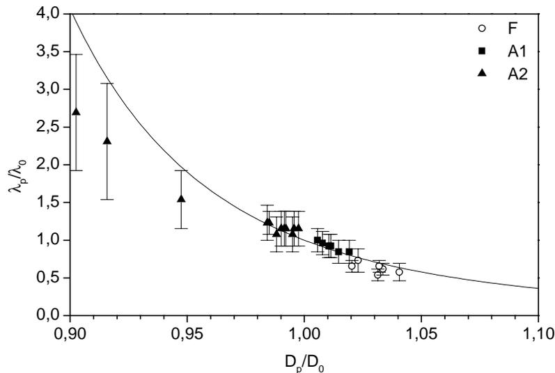
Fig.3 - Dependence of the detonation cell width on the ratio between the detonation velocity of the mixture with aluminium particles  $D_p$  and the pure gaseous mixture  $D_0$ .
