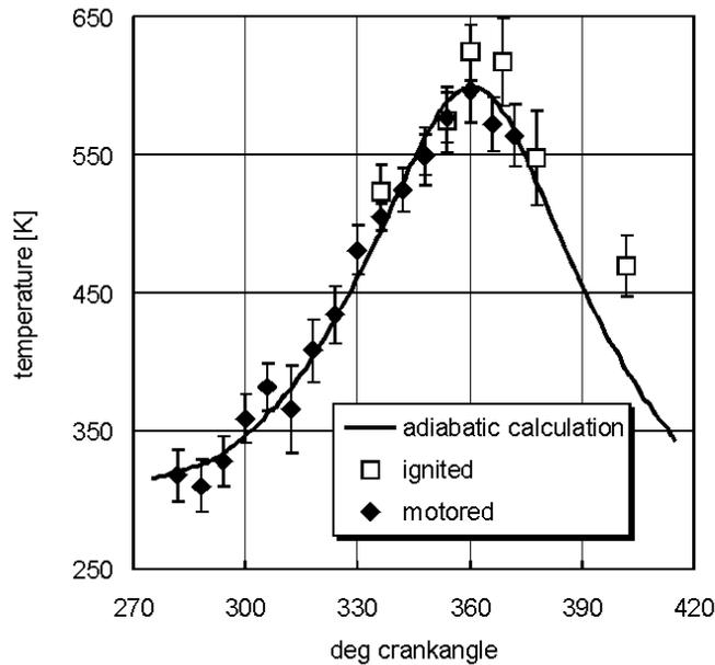
**Figure 5:** Averaged measured temperatures in motored and fired engine cycles, compared to the adiabatic temperature in the motored engine derived from the measured pressure trace with  $\kappa = 1.33$
