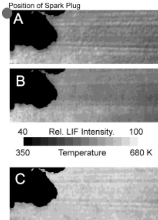
**Figure 3:** Instantaneous tracer-LIF distributions obtained from 3-pentanone after excitation at a) 308 nm and b) 248. c) shows the instantaneous temperature field for a single engine cycle at 360°ca inferred from a) and b). Displayed is a region of 1.9 x 5.4 cm<sup>2</sup>.
