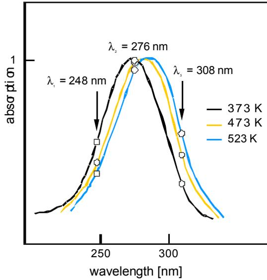
**Figure 1:** Shift of the absorption spectra of 3-pentanone with temperature
