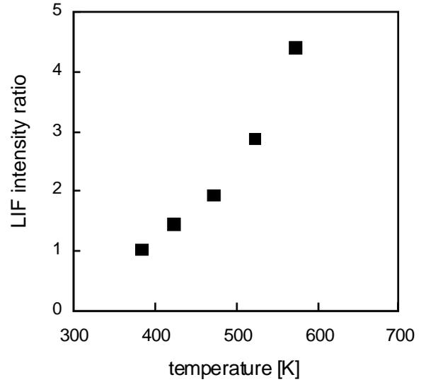
**Figure 2:** Temperature dependence of the ratio  $I_{308} / I_{248}$  of the LIF signal intensities after excitation at 248 nm and 308 nm, obtained in a static cell [4]
