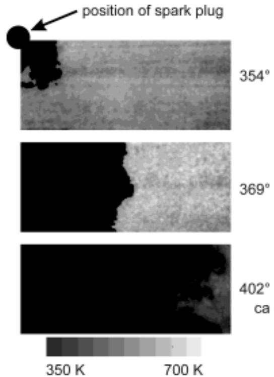
**Figure 4:** Single-shot temperature fields for three different crank angle timings (360°ca is top dead center in the power stroke). The dark area represents burned fuel.
