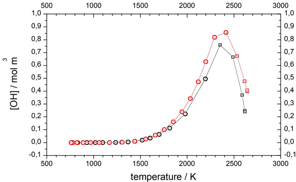
**Figure 3** Correlation between the mass fraction of OH radicals and temperature. This analysis is based on an ensemble of stretched flames calculated for a pressure of 18 bar. Circles mark data obtained in front of the flame front, squares indicate data taken from the post flame region.
