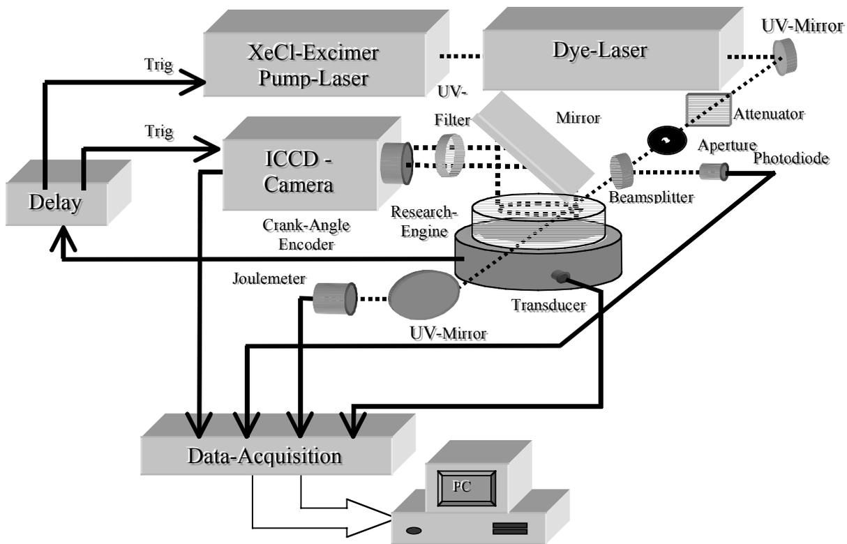
**Figure 1** Experimental set-up of quantitative OH measurements in the combustion chamber of a two stroke engine
