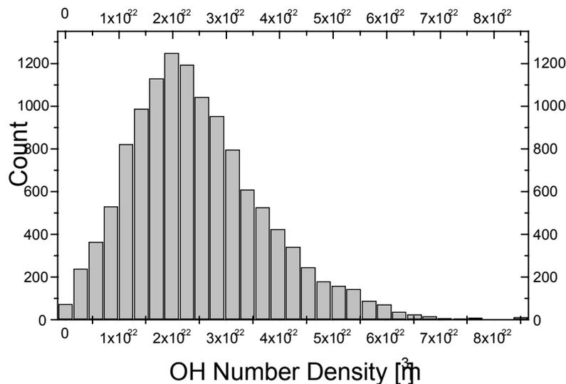
**Figure 2** *Probability density function (PDF) of the OH number density in the burnt gases of an operating IC engine. 20000 data points were used for this graph which all were recorded during the expansion stroke at pressures between 17 and 19 bar.*
