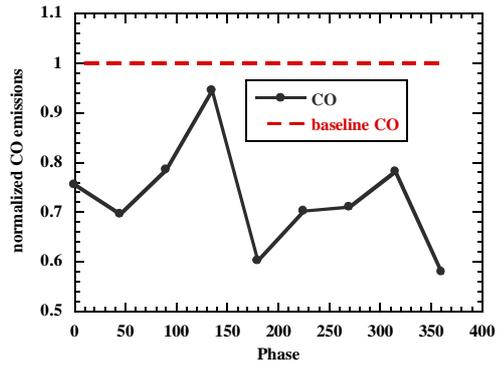
Figure 6: CO emissions as a function of phase in a closed loop controller with antisymmetric pulsed fuel injection (amplitude  $F/F_{max} = 50\%$ ).
