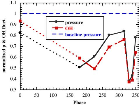
Figure 3: Effect of Phase variation on pressure and OH fluctuations suppression in a closed loop controller with antisymmetric pulsed fuel injection (amplitude  $F/F_{max} = 95\%$ ).
