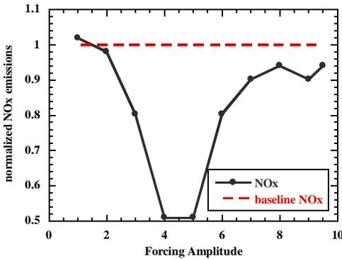
Figure 5:  $\text{NO}_x$  emissions as a function of amplitude in a closed loop controller with antisymmetric pulsed fuel injection (phase=330 deg.).
