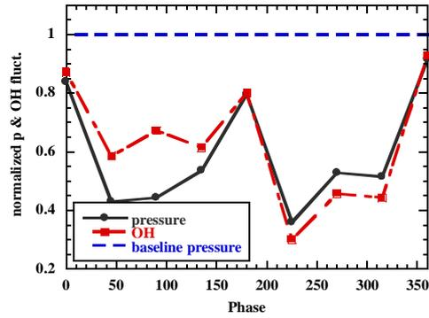
Figure 4: Effect of Phase variation on pressure and OH fluctuations suppression in a closed loop controller with antisymmetric pulsed fuel injection (amplitude  $F/F_{max} = 50\%$ ).
