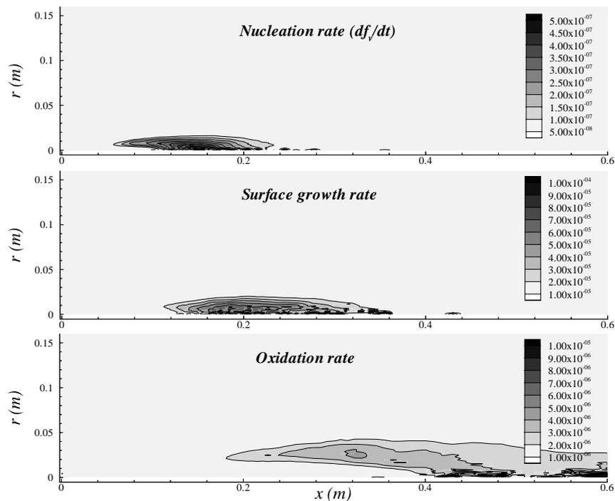
**Fig 5.** Mean soot production rates inside the flame
