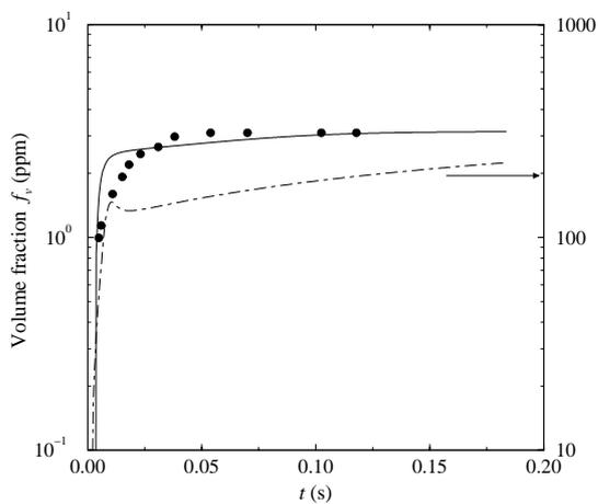
**Fig 1.** Soot volume fraction and particle diameter profiles for the flame of Bonig et al at  $P = 10$  bar
