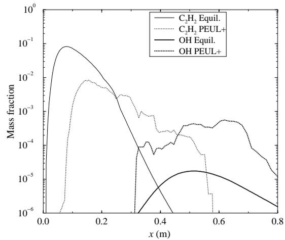
**Fig 4** :  $C_2H_2$  and OH mass fractions on the jet centerline computed with PEUL+ compared to the equilibrium assumption
