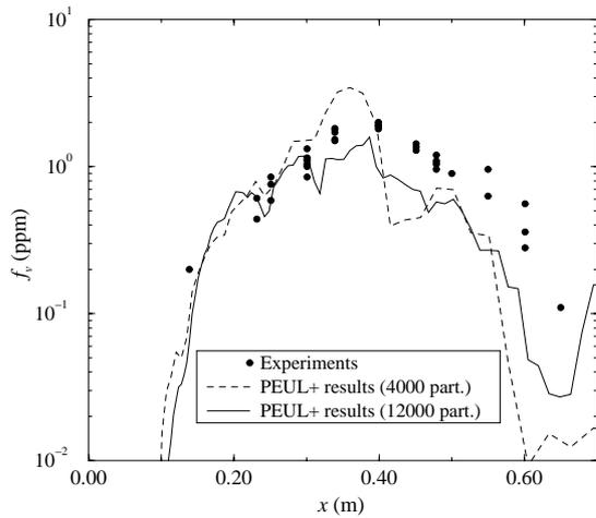
**Fig 3** : Soot volume fraction profiles on the jet centerline
