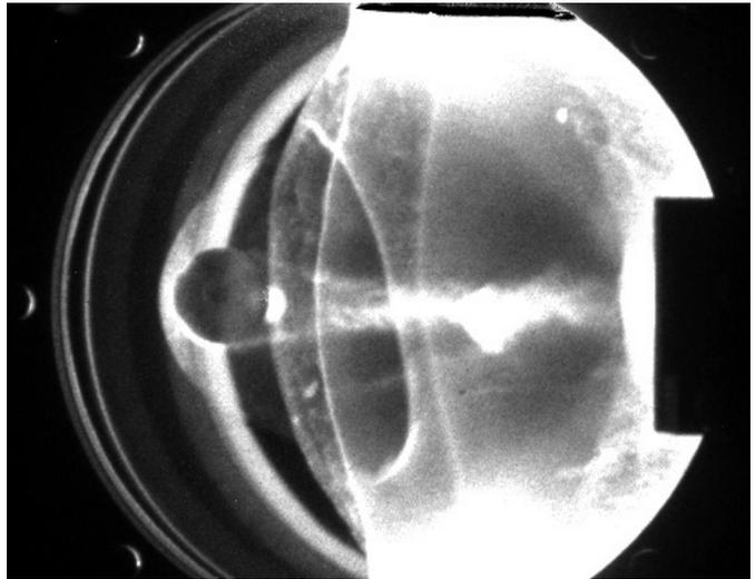
Figure 3: Shot 1832 ICCD:  $\text{C}_2\text{H}_4+3\text{O}_2+4.3\text{N}_2$  at 0.350 bar, 2400 m/s
