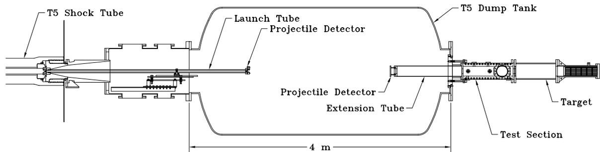
Figure 1: T5 dump tank showing launch tube, test section, extension tube, and target section
