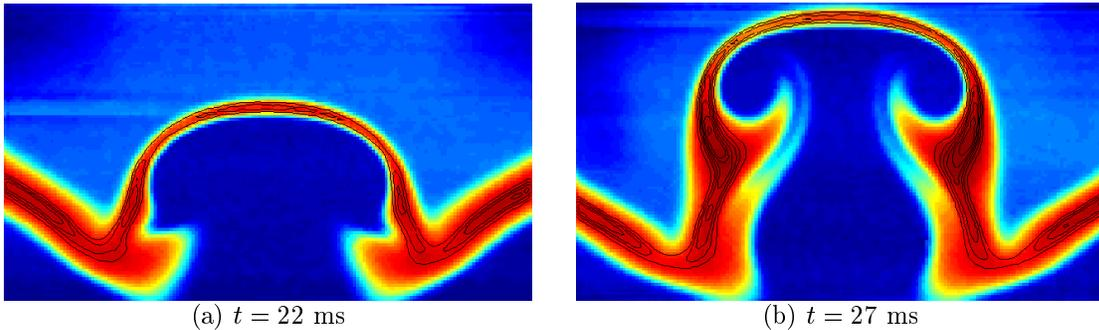
Figure 5: Typical example of simultaneous visualization of temperature field (field of Rayleigh scattering) and flame front position (isolevels of OH PLIF).
