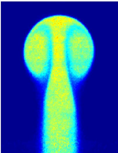
Figure 2: The vortex ring evolves into a starting jet.
