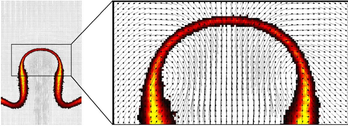
Figure 4: Typical example of simultaneous visualization of velocity field (PIV) and flame front position (OH PLIF).
