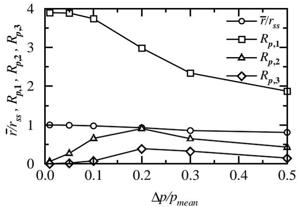
Fig 6 Effect of amplitude of pressure oscillation ( $\Delta p$ ) on response function
