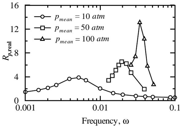
Fig 5 Effect of mean pressure ( $p_{mean}$ ) on the real part of response function
