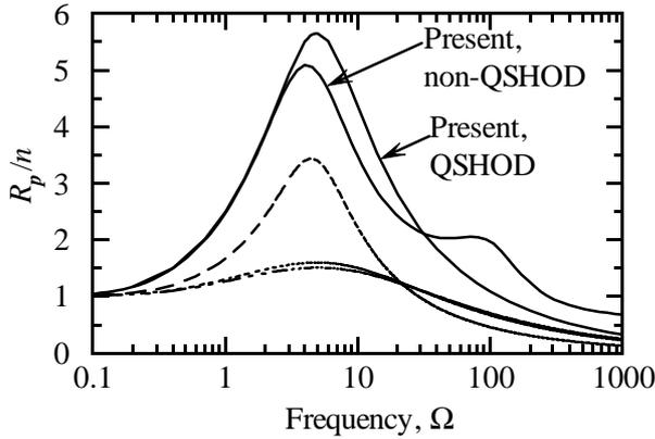
Fig 3 Comparison with linear, QSHOD results of DeLuca [4] and others
